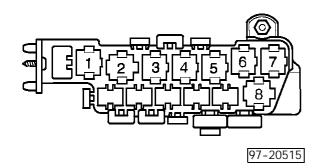
Relay location on the thirteen position auxiliary relay panel, above relay panel:
