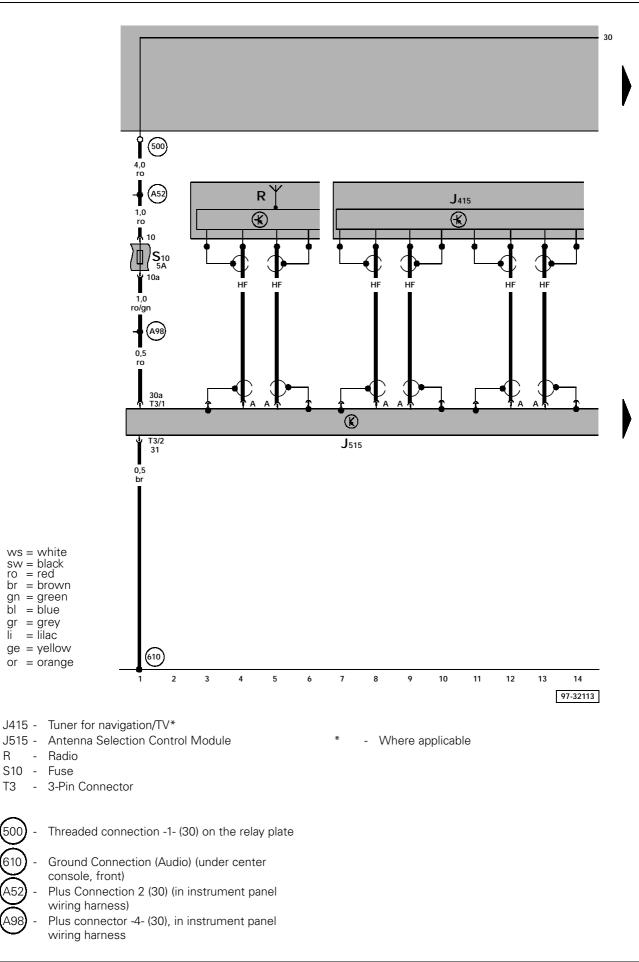
Antenna Selection Control Module, Tuner for navigation/TV, Radio
