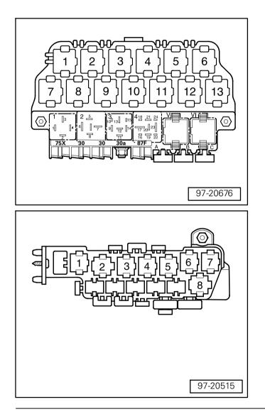
Relay location on the thirteen position auxiliary relay panel, above relay panel:
