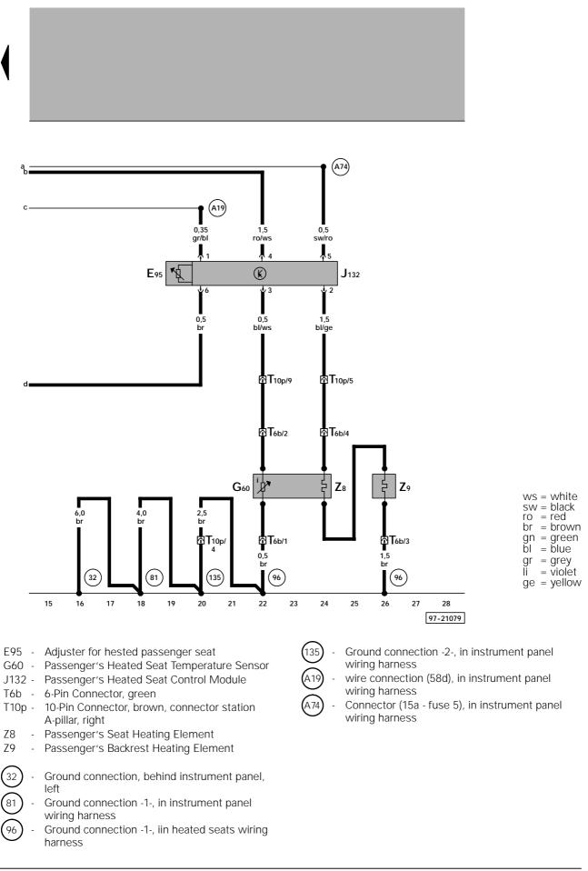
Passenger's heated seat control module, temperature sensor, passenger's seat heating element, passenger's backrest heating element
