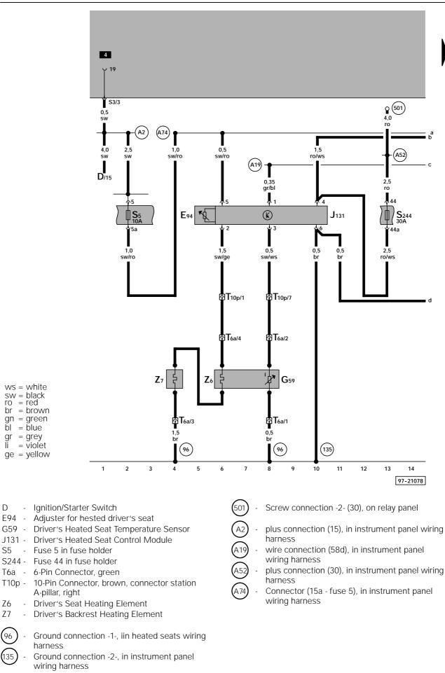
Driver's heated seat control module, temperature sensor, driver's seat heating element, driver's backrest heating element
