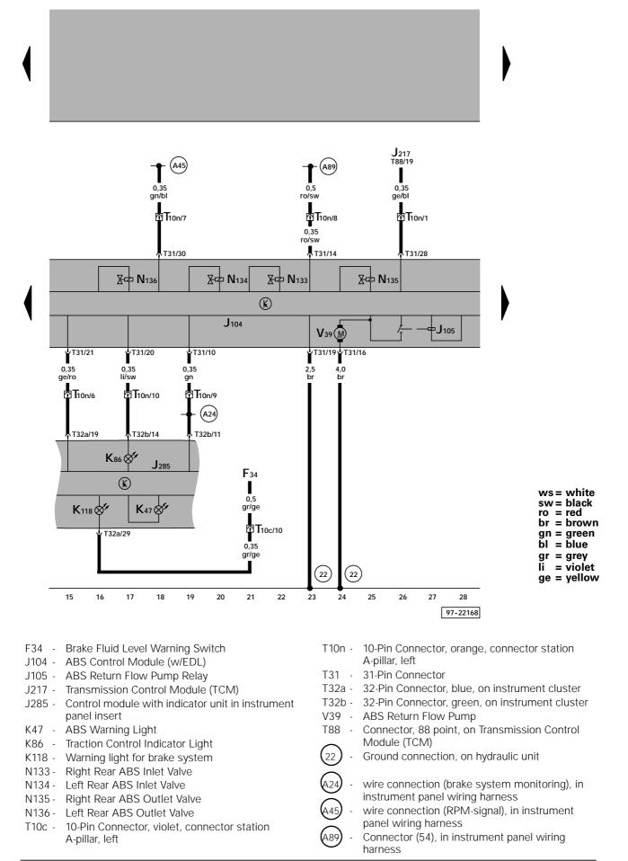
Edition 12/97 USA.5062.03.21 ABS control module (with EDL), ABS return flow pump, ABS warning light, traction control indicator light, Warning light for brake system
