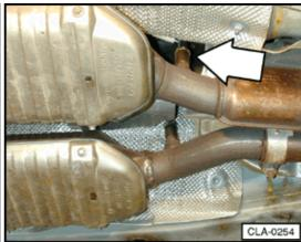
Z30 Heater for Lambda-probe 2 (2.8 ltr. engine)
