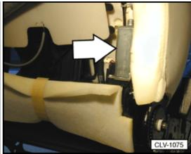
V45 Motor for seatback adjustment, driver seat
