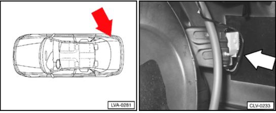
V155 Motor for fuel tank lid unlock
