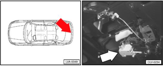
V151 Motor for remote unlock rear lid
