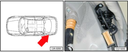
V144 Leak detection pump
