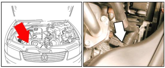
N79 Positive Crankcase Ventilation (PCV) Heating Element
