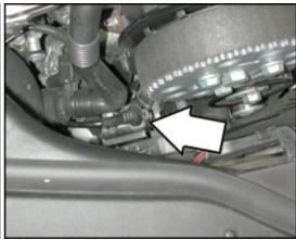
N75 Wastegate Bypass Regulator Valve (2.0 ltr. tdi engine)
