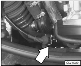
N75 Wastegate bypass regulator valve (1.8 ltr. engine)
