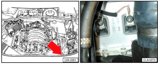
N39 Coolant Fan Control (FC) series resistance
