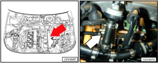
N249 Recirculating valve for turbocharger (1.8 ltr. engine)
