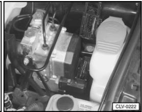
N166 Right front traction control switch-over valve
