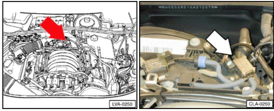
N156 Intake Manifold Tuning (IMT) valve, change over valve (2.8 ltr. engine)
