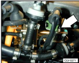
N112 Secondary Air Injection (AIR) solenoid valve (1.8 ltr. engine)
