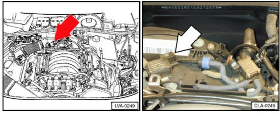
N112 Secondary Air Injection (AIR) solenoid valve (2.8 ltr. engine)
