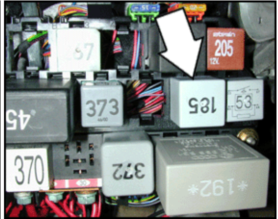
J433 Locking Relay for Starter (anti-theft immobilizer)
