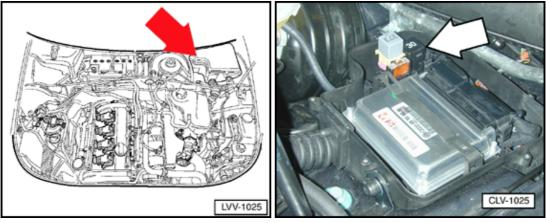
J271 Motronic engine control module (ECM) power supply relay
