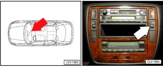
J132 Passenger's heated seat control module
