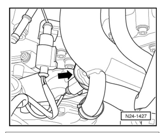
**G62 - Engine Coolant Temperature (ECT) Sensor**
