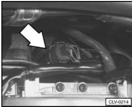
G62 **Engine Coolant Temperature (ECT) sensor (1.8 ltr. engine)**
