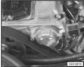
G40 Camshaft Position (CMP) sensor (1.8 ltr. engine)
