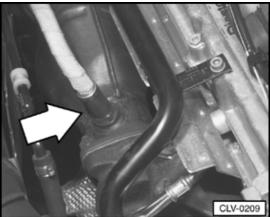
G39 Heated Oxygen Sensor (HO2S) (1.8 ltr. engine)
