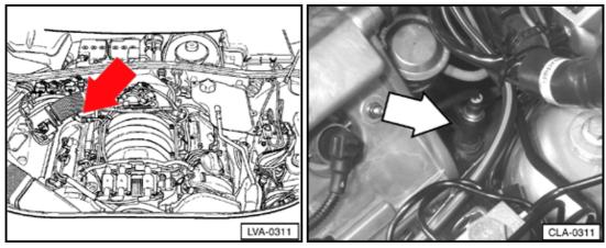
G39 Heated Oxygen Sensor (HO2S) (2.8 ltr. engine)
