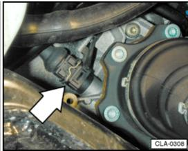
G38 Transmission Vehicle Speed Sensor (VSS)
