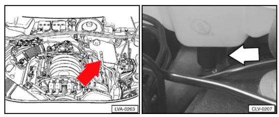
G32 Engine Coolant Level (ECL) sensor
