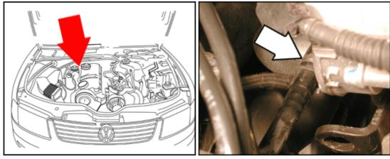
G2 Engine Coolant Temperature (ECT) Gauge Sensor (2.0 ltr. tdi engine)
