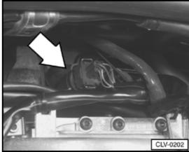
G2 Engine Coolant Temperature (ECT) sensor (1.8 ltr. engine)
