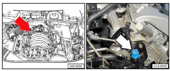
G2 Engine Coolant Temperature (ECT) sensor (2.8 ltr. engine)
