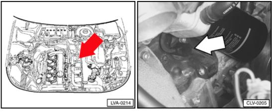
G28 Engine Speed (RPM) sensor (1.8 ltr. engine)
