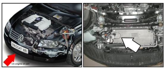
G266 Oil Level Thermal Sensor (4.0 ltr. engine)
