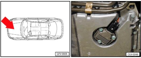
G266 Oil Level Thermal Sensor (2.8 ltr. engine)
