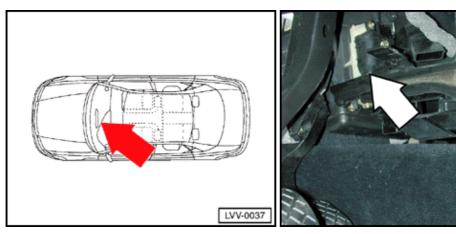
G192 Sender for outlet temperature, floor outlet
