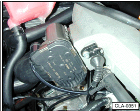
G187 Angle sensor –1– for throttle drive (power accelerator actuation) (1.8 ltr. engine)
