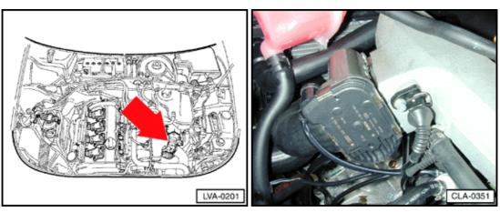
G186 Throttle drive (power accelerator actuation) (1.8 ltr. engine)
