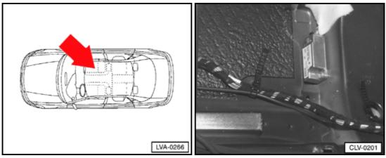
G180 Crash sensor for side airbag, passenger side
