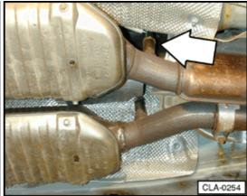
G131 Oxygen sensor (O2S) 2, behind Three Way Catalytic Converter (TWC) (2.8 ltr. engine)
