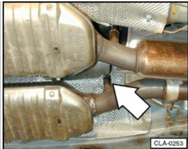
G130 Oxygen sensor behind Three Way Catalytic Converter (TWC) (2.8 ltr. engine)
