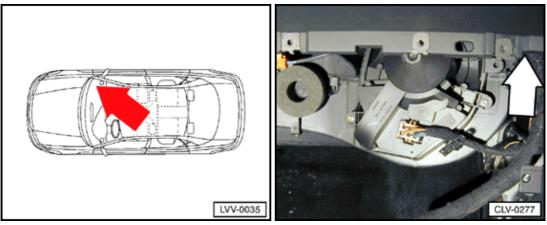
G113 Back pressure flap motor position sensor
