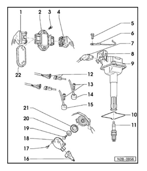
Ignition system components, removing and installing
