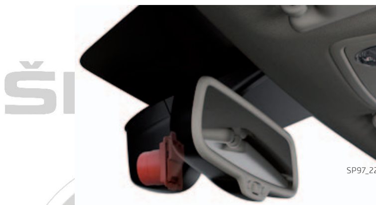
Separate camera of the Distance Light Assistant - FLA
