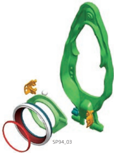
new assembly of the lever on clutch K1* (as of 01.06.2011)
