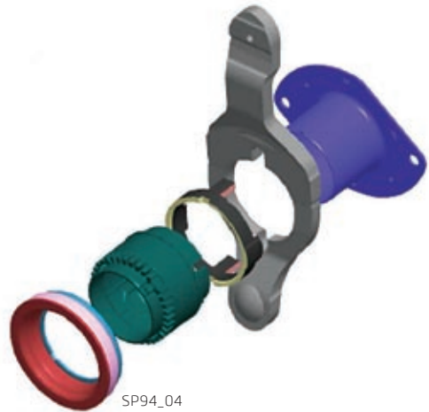
new assembly of the lever on clutch K2* (as of 01.06.2011)
