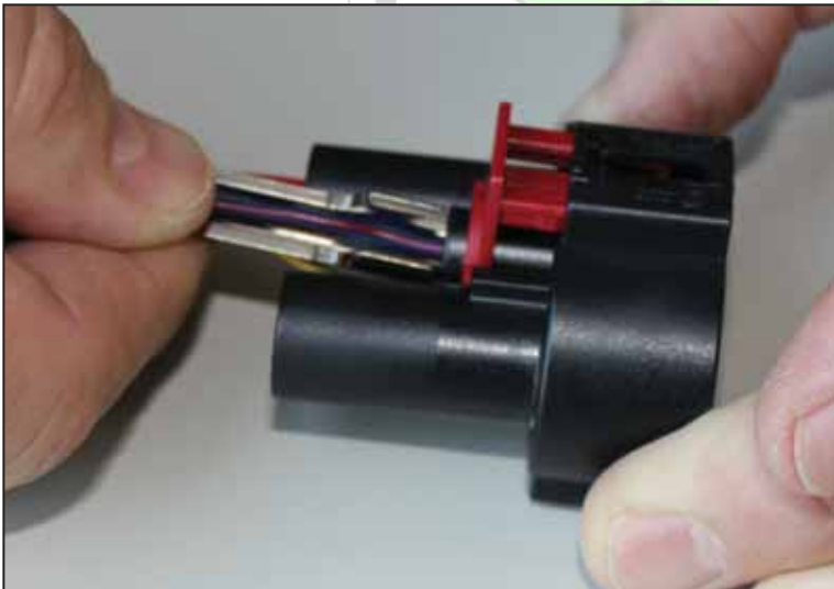
Pressing the seal into the terminal strip (up to the stop)
