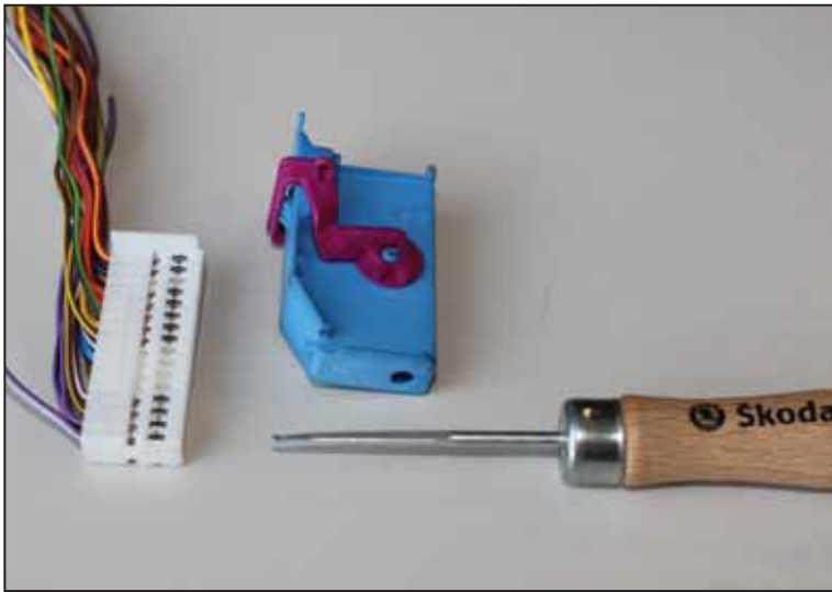
e) Removing the terminal strip with plug connectors after releasing the secondary fuse (stop)
