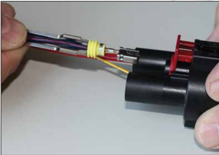
Inserting the conductor with seal in the assembly device
