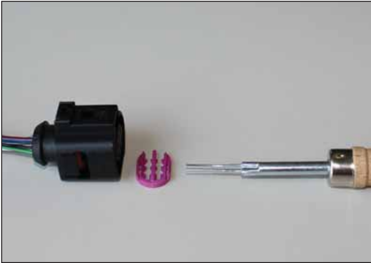
d) Releasing the secondary fuse
