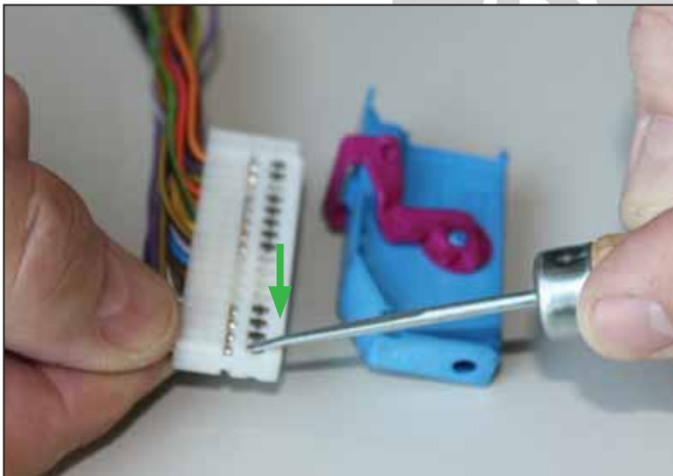
Releasing the plug connector with the prescribed tool
