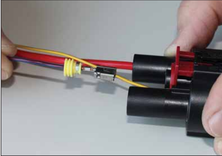
c) Conductor with plug connector and seal ready for installation
