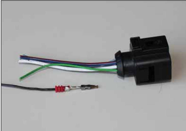
a) Conductor with plug connector and seal ready for installation
