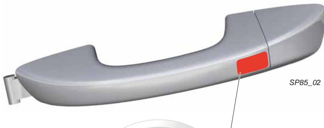
Surface of the capacitive sensor for locking the vehicle
