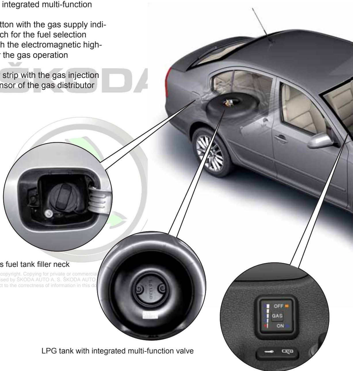
Conversion button with the gas supply indicator and the switch for the fuel selection
