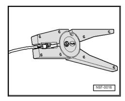
Crimp the stripped ends of the repair wire and single cable of the vehicle's wiring loom with the crimping pliers and a crimp connector, as described in section ⇒ b2.9 reak with single repair point", page 66
