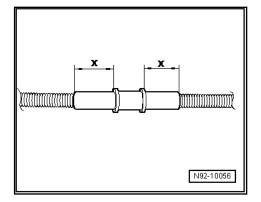
Slide the shrink hose -5- over the corrugated pipe and connect up the connecting pieces -2- and -3-.
