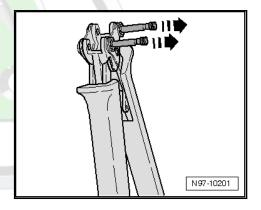
Insert the required tool head from above -arrow- into the pliers handle.
