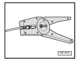
Crimp the stripped ends of the repair wire and single cable
