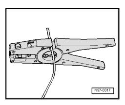
Strip the ends of the repair wire and the vehicle's single cable by 6-7 mm with the wire stripper.
