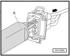
Cut off the old contact with single cable seal from the vehicle's wiring loom.
