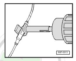
Heat the crimp connector with the hot-air blower lengthways from the centre to the outside until it is completely sealed and the adhesive is coming out at the ends.
