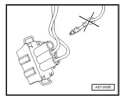
Slide the repair wire with the new contact into the correct chamber of the socket housing -arrow- until it locks into place.
