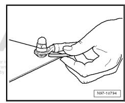
Hold the injector above the cable eye and spray all around the bolt and the cable eye. Citigo 2012 ➤, Citigo-e iV 2020 ➤, Enyaq 2021 ➤, Enyaq Coupe 2021 ➤, Fabia 2000 ... Electrical System - general notes - Edition 12.2021
