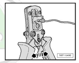
Slide the single cable seal in the direction of the stripped end of the wire until it is sealed flush with the wire insulation (see Fig.).
