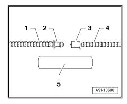
Secure the repair point with the shrink hose.
