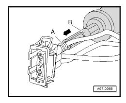
Shorten the repair wire and single cable of the vehicle's wiring loom as required with the wire stripper -VAS 1978/3-.
