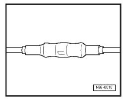
Expose the wire to be repaired (approx. 20 cm to each side of the repair point).
