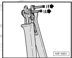
Insert the required head adapter from above -arrow- into the base body of the crimping pliers.
