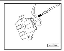
Slide the single cable seal -A- onto the free end of the repair wire -arrow-.
