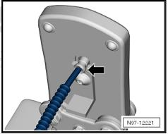
Open the optical fibre pliers and remove the optical fibre with brass pin contact.
