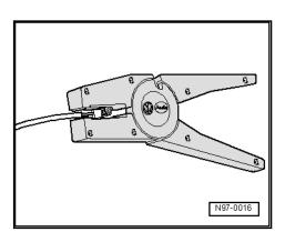
Slide crimp connectors onto the two stripped ends of the vehicle's single cable and crimp them with the crimping pliers.
