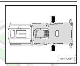
Slacken the tensioning sleeve of the socket -1- out of the catch peg -2-, tilt out the tensioning sleeve -arrow- and remove it.
