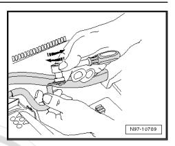
Check the burr on the cable eye and remove with the reamer if necessary.
