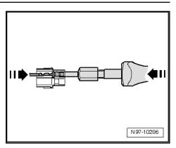
Take the contact on the wire and press it gently into the socket housing -arrow-.
