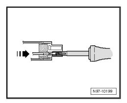
Guide the correct release tool for the socket housing into the unlocking channel on the socket housing.
