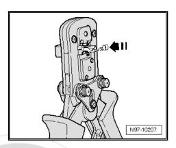
Insert the stripped end of the wire with the positioned single cable seal into the crimp contact -arrow- until it lies against the "wire stop".
