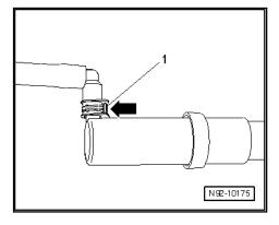
In order to connect, press together the connections until they lock audibly. Check for secure locking by pulling at the connection.
