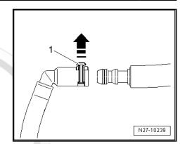
In order to connect, press together the connections until they lock audibly. Check for secure locking by pulling at the connection.
