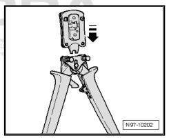
Lock the tool head in the pliers handle by pushing in the pins -arrows-.
