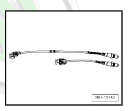
Fix the excess length of the unit probe (approx. 50 - 250 mm) by tying it back to the length of the cable ties -1-.
