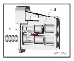
Unlock the secondary lock -2- with a small screwdriver and remove the optical fibre.
