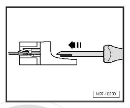
A selection of release tools is part of the wiring loom repair set -VAS 1978 B- and previous sets.
