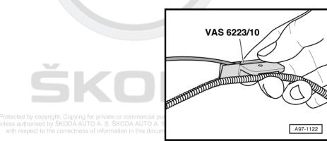
Place the corrugated tube assembly pliers on the slit in the corrugated tube.
