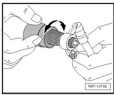
The battery poles are cleaned with rotary movements using the bottom side of the battery pole cleaner.
