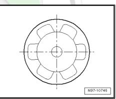
Only used for LSF Lambda probes- 4-pin. Variant D2, 6 openings each 2 mm
