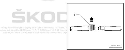
In order to connect, press together the connections until they lock audibly. Check for secure locking by pulling at the connection.
