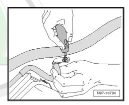
Position again the cable eye and screw on to the recommended tightening torque.
