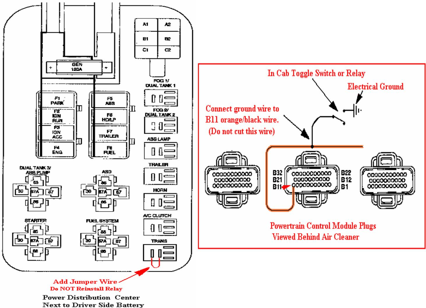
**NOTE: Some Rams have the TRANS relay located in a different position than shown in the above diagram. Consult the diagram on the underside of your PDC cover to determine the exact location of your TRANS relay.**
